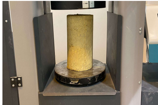
Material Research (rammed earth) Testing soil mixture, Lab compressive test
