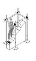
Protection for Rammed earth wall
